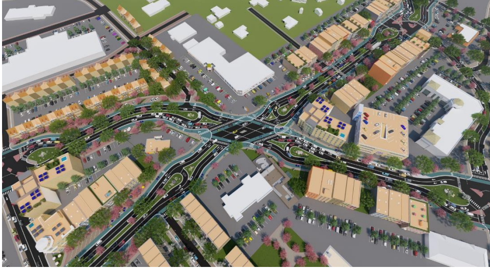
Figure 2-11 Conceptual rendering of a Bowtie/Teardrop Intersection with U-turn close to main intersection
