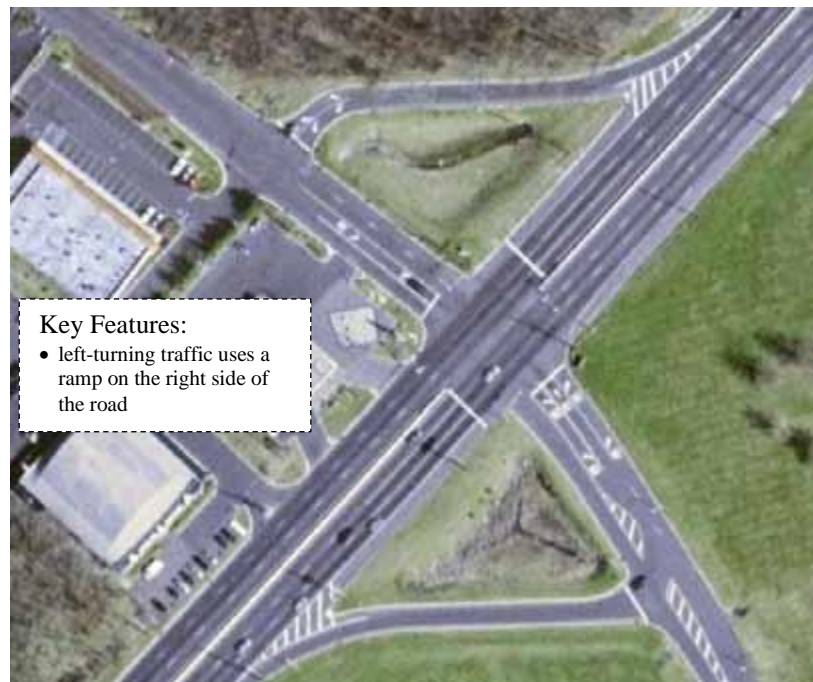
Figure 2-24 A Typical jughandle intersection in New Jersey
