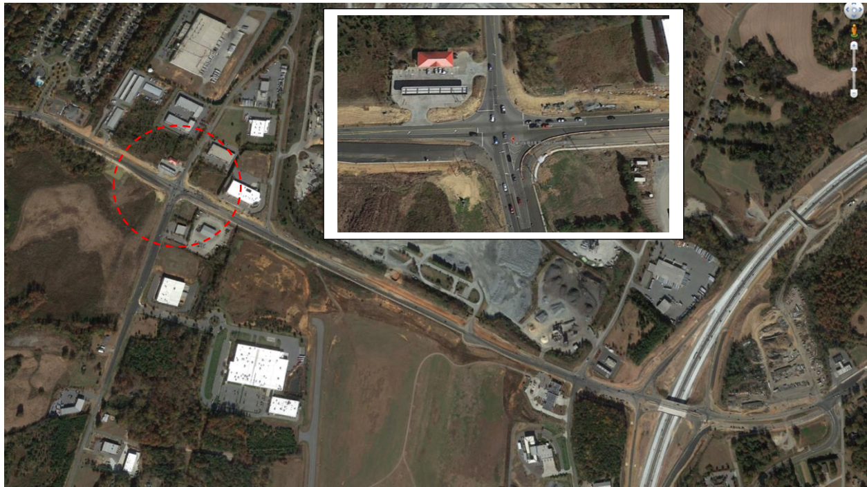
Figure 5-7 Aerial view of the Poplar Tent Rd and Derita Rd Median U-Turn Intersection in Concord, NC
