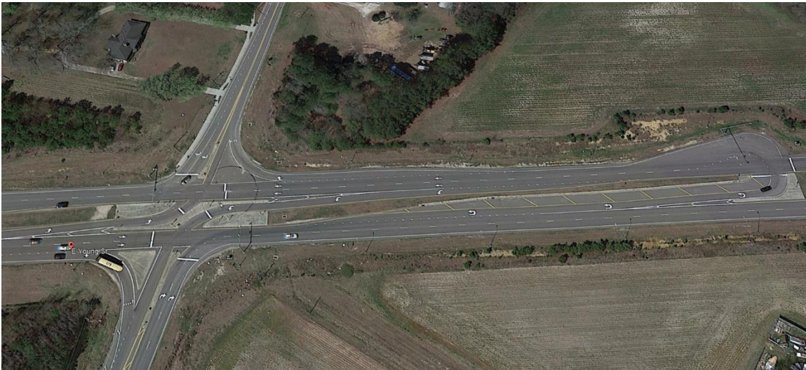
Figure 5-13 US 401 and Young St. Signalized Restricted Crossing U-Turn Intersection in Wake Forest, NC
